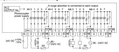
Terminal blocks are not equipped with built-in fuses. In order to prevent breakdown of circuits caused by load short-circuit, provide a fuse of 5 to 10 A for every four points.
